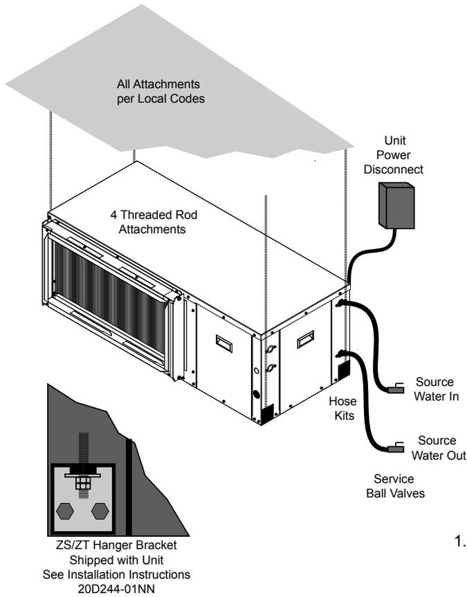
**Note:** Hanger shown in the preferred locations, but may be assembled to side of the unit as necessary.
