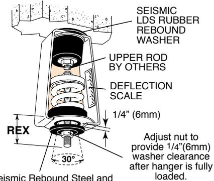
Seismic Rebound Steel and Bonded LDS Rubber Washer holds precompression and limits upward seismic motion. Hangers are precompressed to rated load or assigned load as required. Scale indicates deflection.
