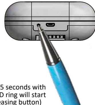
Depress button for 5 seconds with a ball point pen (LED ring will start spinning after releasing button)
