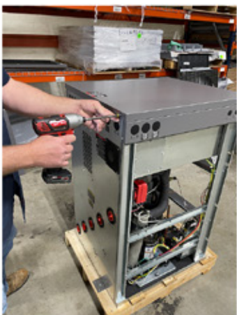
To remove the top, take the two screws out of the rear of the unit.
