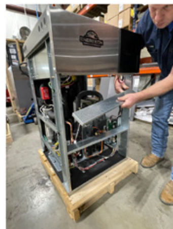
Remove the center Braces (x2, 8 screws).
