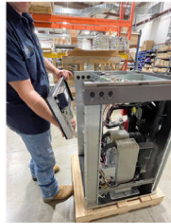
Remove the front HMI Panel.
