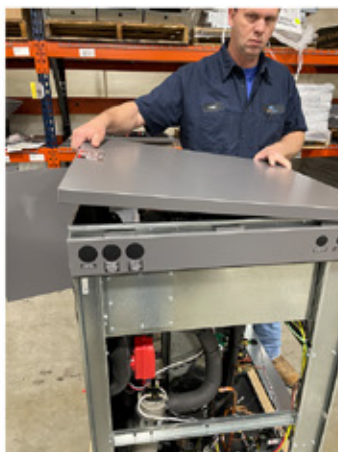
Slide the top towards the rear and remove it.
