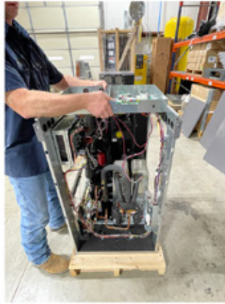
Pull up on the control box and move to the front of the unit.
