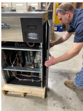
Pull out the front of the panel and slide to the rear.
