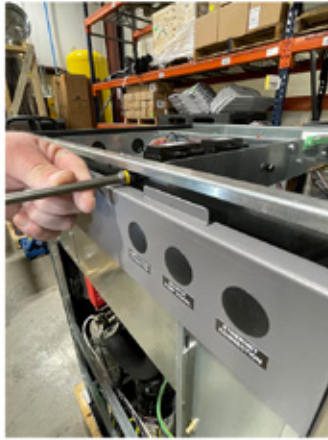
Remove four screws from the control box.
