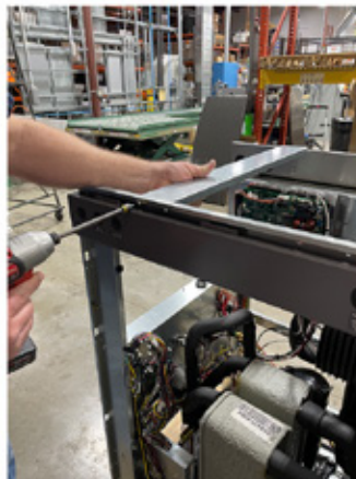
Add the previously removed bracing to the top where the control box was.
