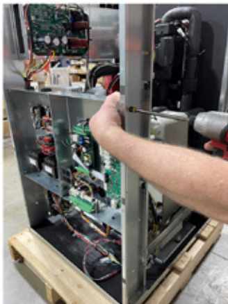
Add four screws into control box on both sides.
