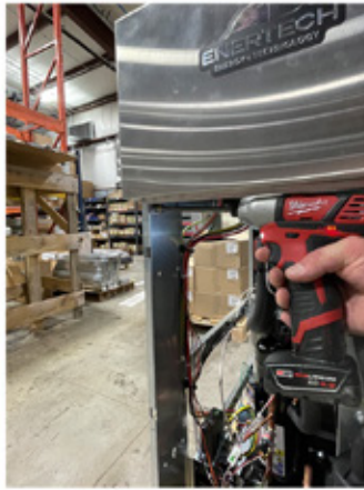
Remove two screws from the front panel/corner post.
