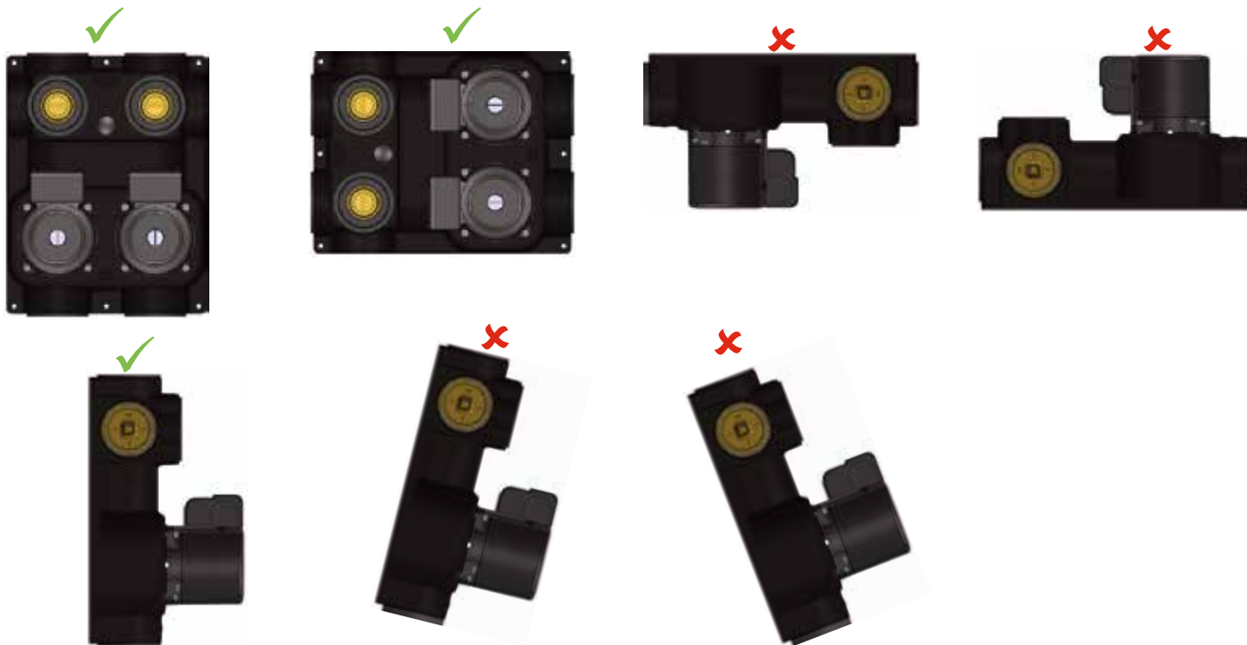
Figure 2: Acceptable mounting positions for Flo-Link and GPM series flow centers.
